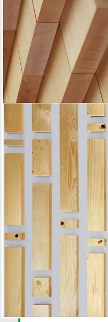
Fixed length cutting Defect cutting Optimisation
